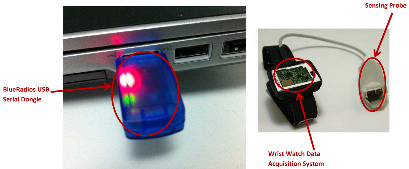
Figure 11 Health Hub Measurement Setup Hardware Description
