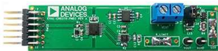
Figure 11: The EVAL-CN0370-PMDZ circuit evaluation board is a complete single supply, low noise LED current source driver that is controlled by a 16-bit DAC, all in a PMOD form factor. (Image source: Analog Devices)
