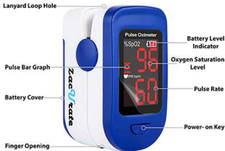
Figure 1: The patient places a finger inside this portable pulse oximeter to get a clear indication of pulse oxygen level and heart rate. (Image source: Zacurate)
