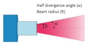
The BPP value of the laser beam delivered from a fiber optic cable is given as the product of fiber core radius and output divergence angle (half angle). Smaller fiber core radius and/or smaller output divergence angle give a better beam quality (lower BPP-value).
