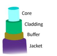
In an optical fiber the part with the higher reflective index is called the "core" and the material, with lower reflective index, surrounding the core, is called the "cladding". For high power applications, only fibers with a core made of pure fused silica are used. The most common design surrounds the core with a cladding made of doped silica. Outside the cladding, there are at least two more layers to protect the fiber and make it flexible—the "buffer" and the "jacket".
