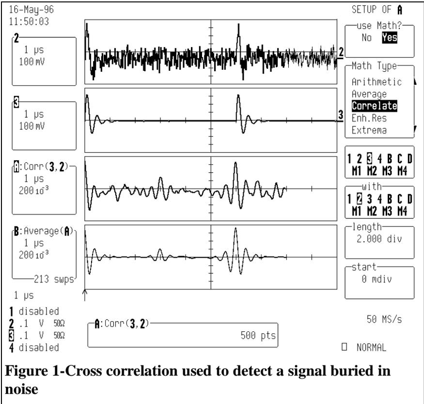
**Figure 1-Cross correlation used to detect a signal buried in noise**
