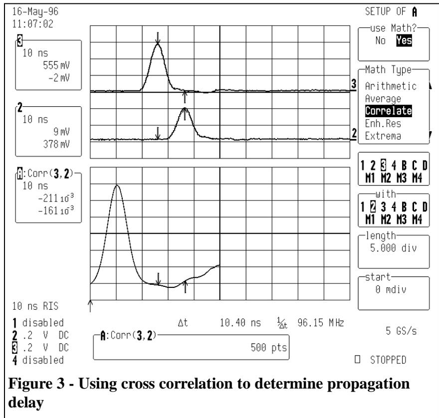
**Figure 3 - Using cross correlation to determine propagation delay**
