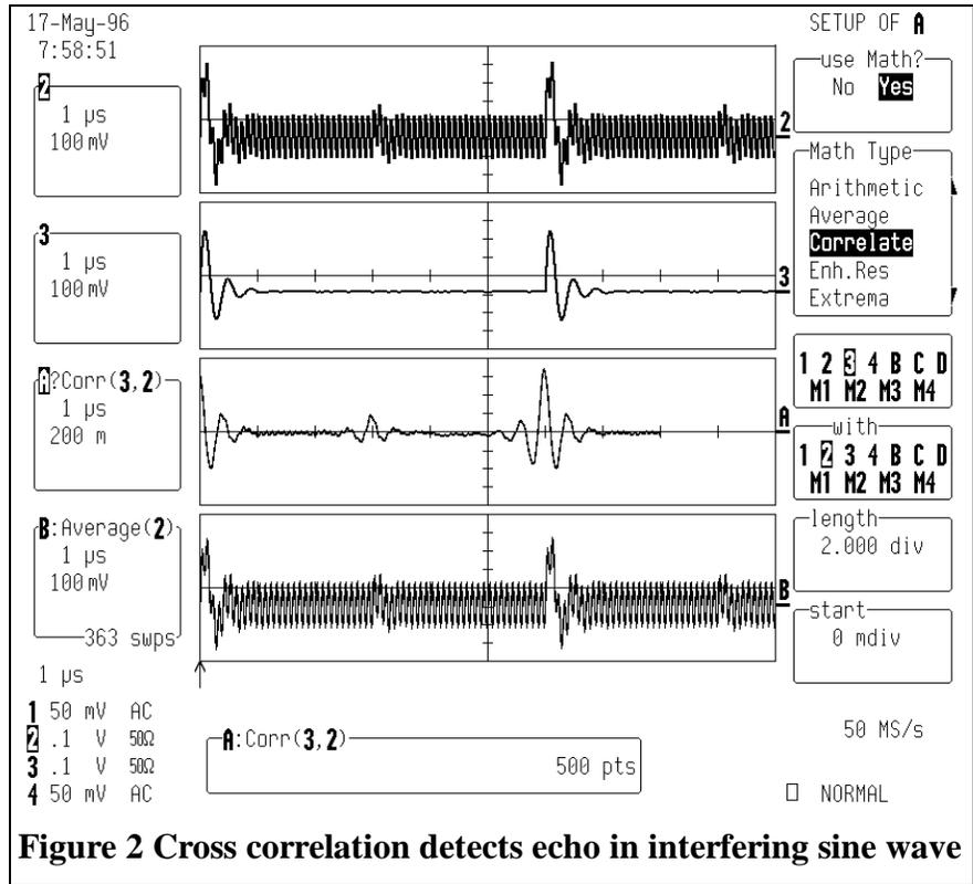
**Figure 2 Cross correlation detects echo in interfering sine wave**
