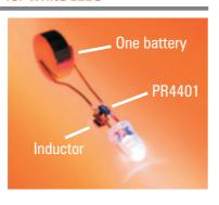
cell. Output currents of 20mA (PR 4401) and 40mA (PR 4402) can be achieved. The only other component needed is an inductor. A cleverly devised control circuit produces a constant output current.
