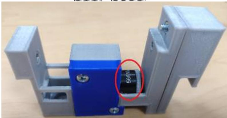
2. The Neutral Density Filter is used to decrease the light intensity for a wide range of wavelengths. For instances wherein the LED light intensity easily saturates the photodiode current input to the ADPD4101 [<https://www.analog.com/ADPD4101>], adding the Neutral Density Filter will help decrease the input current range.
