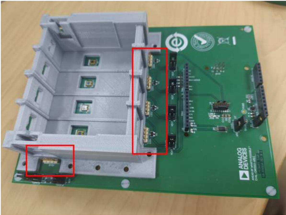
Secure the Mounted Base to the Main Board using 10 S2 Screws and 10 Hex Nuts at the holes at its sides as shown below.
