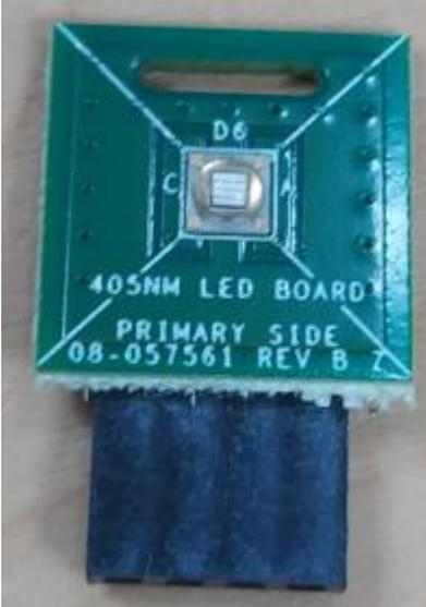
A photograph of a green square LED board with a central square LED chip. The board is labeled with "D6", "405NM LED BOARD", "PRIMARY SIDE", and "08-057561 REV B Z". A blue rectangular component is attached to the bottom edge of the board.  |
