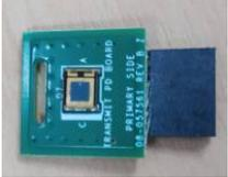
A green PCB with a square photodiode in the center. Text on the board includes "TRANSMIT PD BOARD", "PRIMARY SIDE", and "08-0373561 REV B".    |
