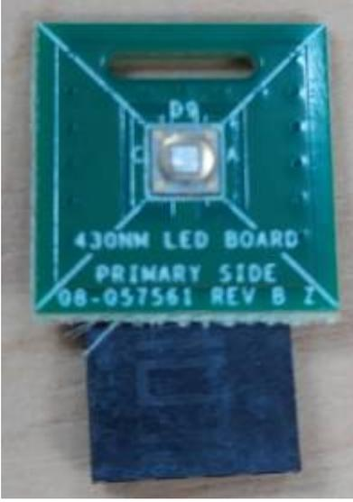
A photograph of a green square LED board with a central square LED chip. The board is labeled with "D9", "430NM LED BOARD", "PRIMARY SIDE", and "08-057561 REV B Z". A blue rectangular component is attached to the bottom edge of the board. |
