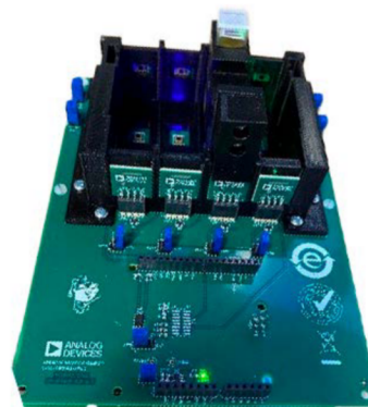
Figure 4. The CN0503 taking a pH measurement.
