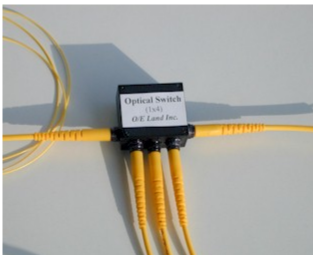
Figure 2. Customer Made 1 x 4 Wide Band Optical Switch
