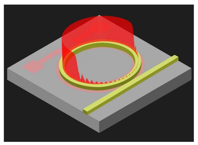
This is an illustration of a microring resonator with an integrated heater
