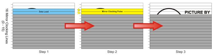
Figure 4-4. Dual Block Mirror Clocking Pulse
