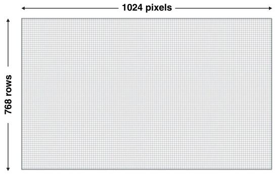
The CMOS memory array consists of 768 rows of 1024 pixels long. 1 = on, 0 = offEach row is randomly or sequentially addressable (automatic counter).
