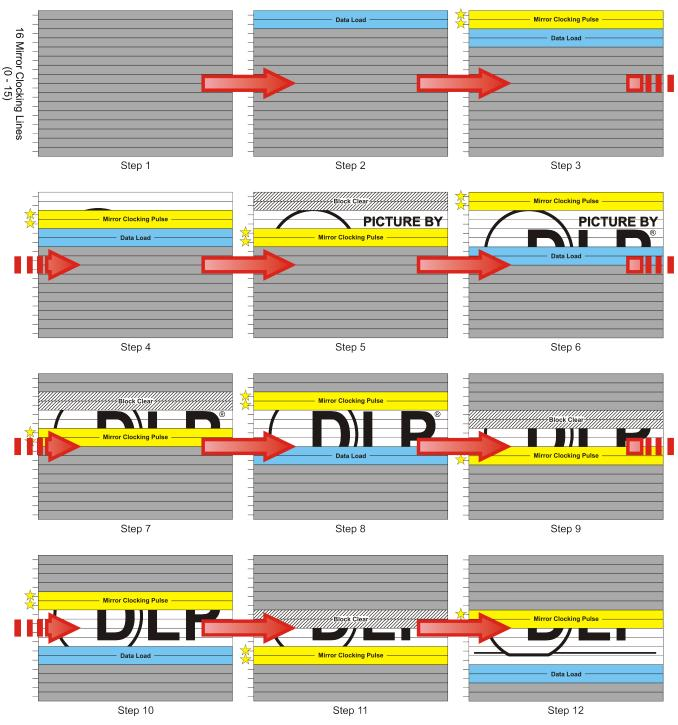
Figure 4-7. Phased Mirror Clocking Pulse Steps
