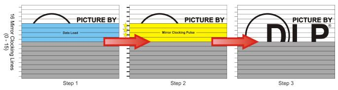
Figure 4-5. Quad Block Mirror Clocking Pulse
