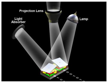
Figure 2-1. Pixels in On and Off State
