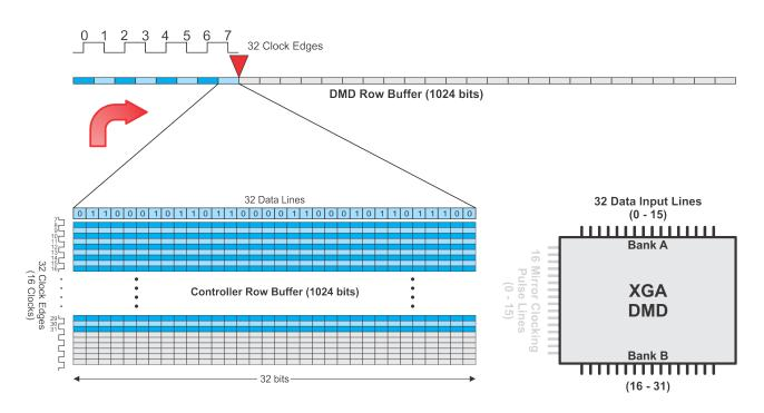
Row data is loaded 32 bits per clock over 32 edges (1024 bits per row) for the 2xLVDS XGA Type A DMD.
