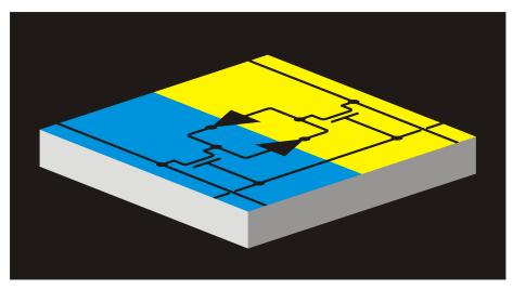
Figure 2-3. Dual CMOS Pixel Memory
