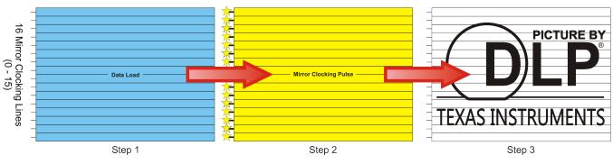
Figure 4-6. Global Mirror Clocking Pulse
