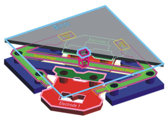
Figure 2-2. Pixel With Labeled Parts
