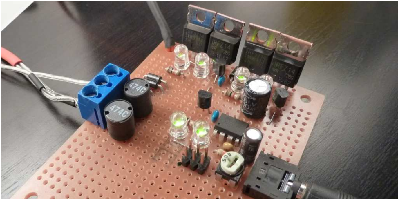
The LEDs are all functionally required - I use them as zener diodes.
